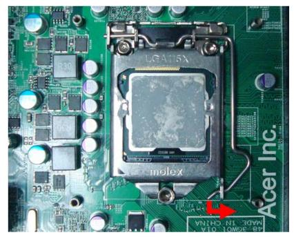
2. Lift the load lever and load plate to the fully open, upright position (1) and (2).
